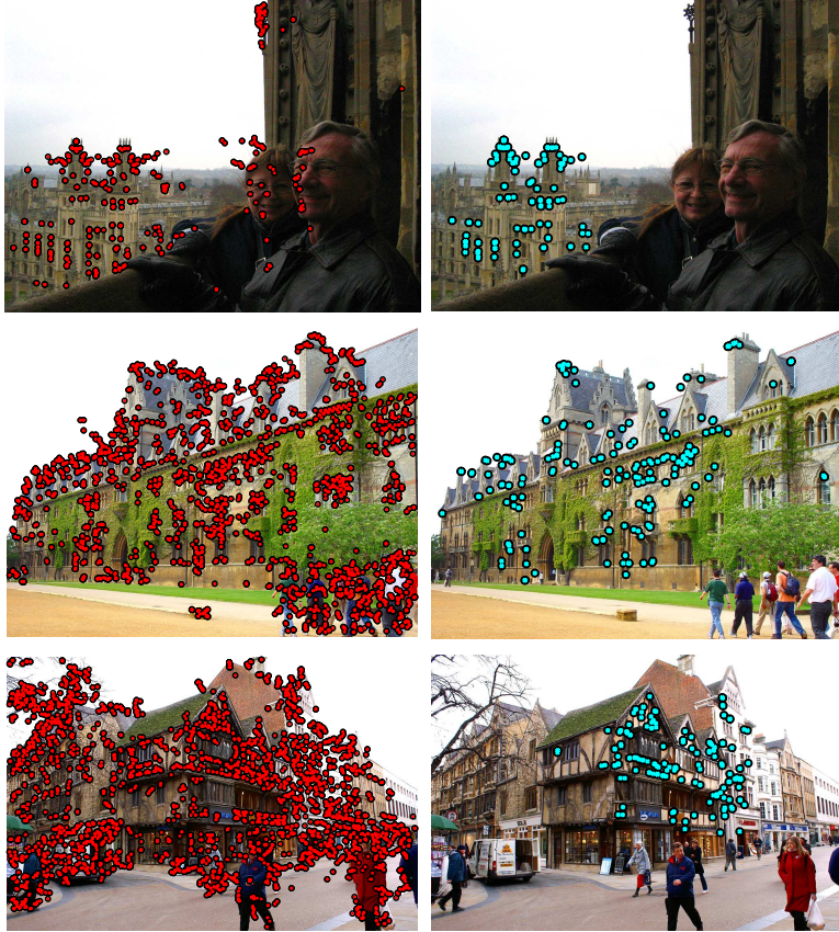
Figure 1.1: Original image features ( left ) and those preserved by robust feature selection ( right ). Transient objects in the foreground and non-distinctive areas of the scenes do not contain robust features.
