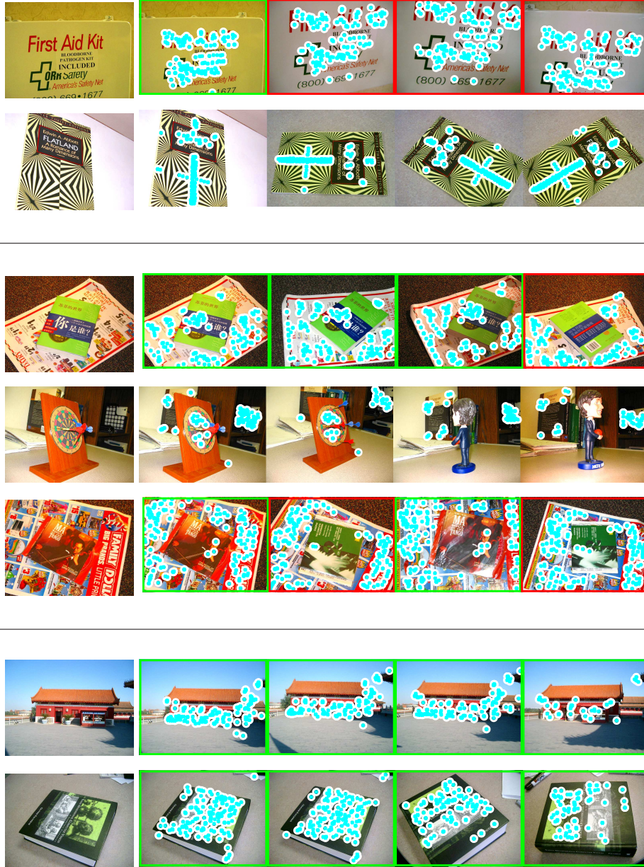
Figure 7.8: Example query images and top 4 matches from the University of Kentucky dataset. Top: Mismatches resulting from challenging objects. While these images contain the same object, they are photographed in different conditions and are labeled as different objects. Middle: Mismatches caused by RFS identifying the background. Bottom: Successful matches.
