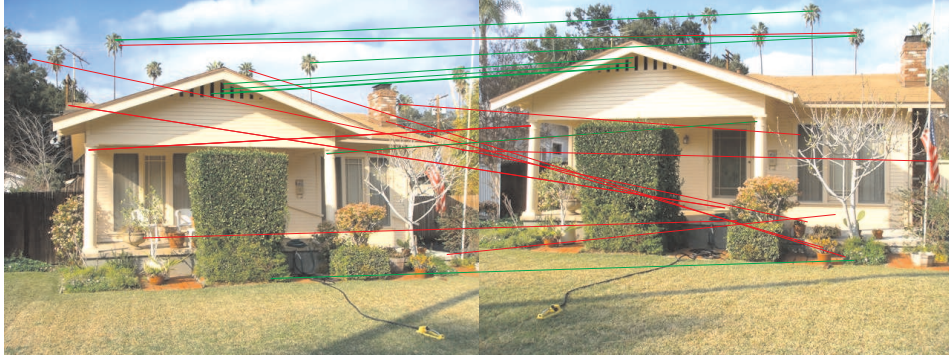
Figure 4.1: Results of geometric verification of traditional descriptor-based feature matching ( top ) where query image features are matched to at most a single database feature (one-to-one). BOW-based feature matching ( bottom ) allows multiple query image features to match multiple database features (many-to-many).
