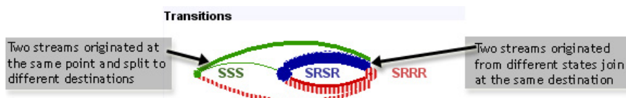
Figure 7.6: Transitions Panel. With S denoting a Search event state and R, a ResultClick event state, the display shows transitions between the pattern S \rightarrow S \rightarrow S , S \rightarrow R \rightarrow S \rightarrow R , and S \rightarrow R \rightarrow R \rightarrow R . The colours of the arcs are user-defined and represent the originating patterns.
