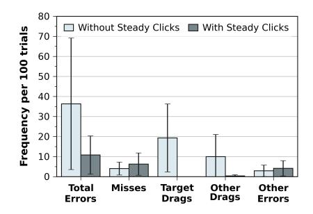
Figure 6.2: Frequency of errors per 100 trials (N = 11). From left to right the bars represent: total errors, misses (i.e., selections of a non-target item), drags on the target item, drags on a non-target item, and other (i.e., clicks outside the target region or blocked clicks). Error bars represent 95% confidence intervals.
