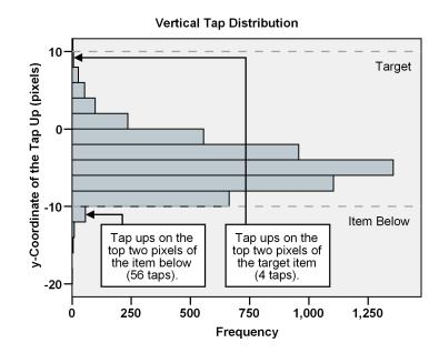
Figure 3.7: Histogram of the vertical tap distribution (for taps on the target item and the item below), relative to the center of the target. (*Bin size* = 2, N = 5127).
