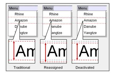
**Figure 4.1:** In a traditional menu, the active target region (shown by dashed lines and arrow) is centered on the text (left); in a reassigned edge menu, it is shifted down by 10% of its height (center); and in a deactivated edge menu, it is reduced by 10%, such that the top region becomes an invisible menu separator (right).
