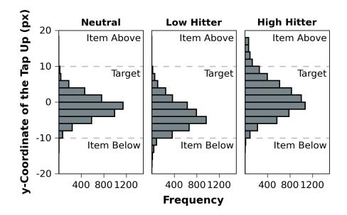
**Figure 4.8:** Histograms of the vertical tap distributions (for taps on the target item and the lower/upper half of the item above/below) for each hitter group and across all interfaces, relative to the center of the target item. (*Bin size* = 2.)
