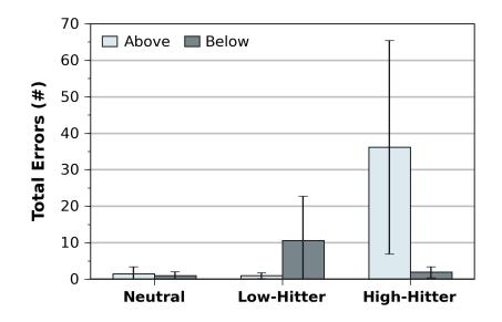
Figure 4.7: Errors above and below the target item (across all interfaces), by tap distribution group (N = 24). Error bars represent 95% confidence intervals.
