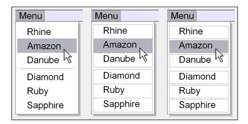
**Figure 4.10:** Proposed visual presentations for the reassigned edge (center) and deactivated edge (right) approaches as compared to a regular menu (left). For the reassigned edge approach, the label is shifted up within the target area. For both approaches, the target boundaries are clearly marked by borders.
