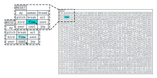
**Figure 6.1:** Screen shot of the evaluation task showing how the target underneath the cursor was highlighted when it was the desired target (upper magnification, cursor on 'flow') and when it was not (lower magnification, cursor on 'cool').
