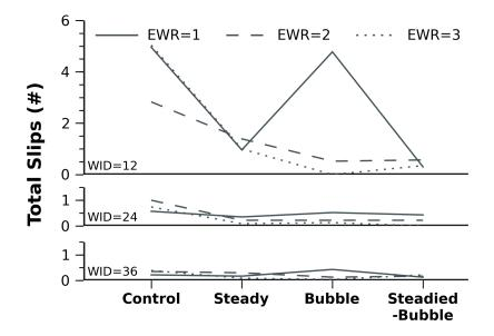
Figure 7.4: Average total slips by CT, WID, and EWR (N = 23, for 36 trials).
