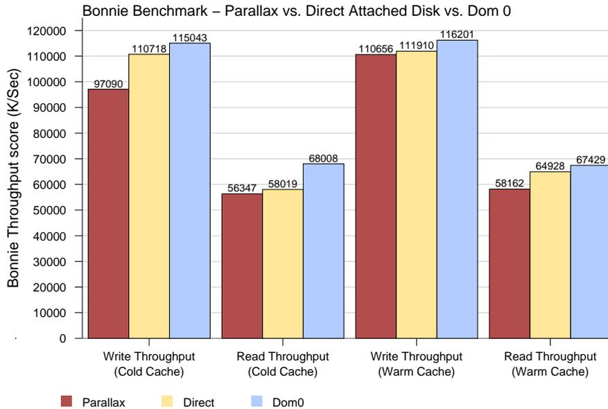
**Figure 5.1:** System throughput as reported by Bonnie++ during a first (cold) and second (warm) run.
