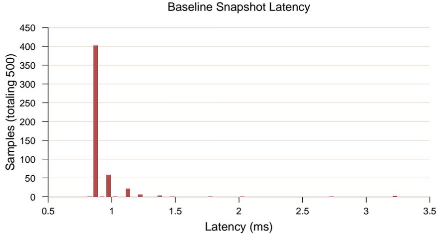
**Figure 5.7:** Snapshot latency of running VM during constant checkpointing.
