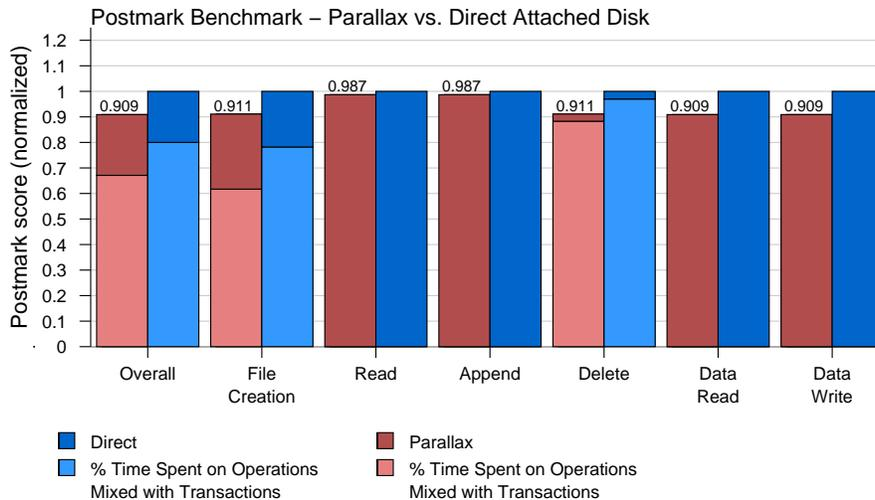
**Figure 5.2:** PostMark results running against network available filer (normalized).
