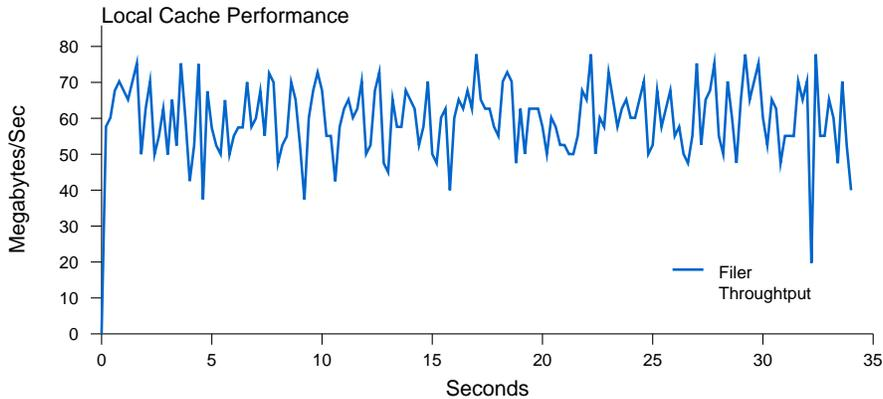
**Figure 5.10:** Performance of bursted write traffic.
