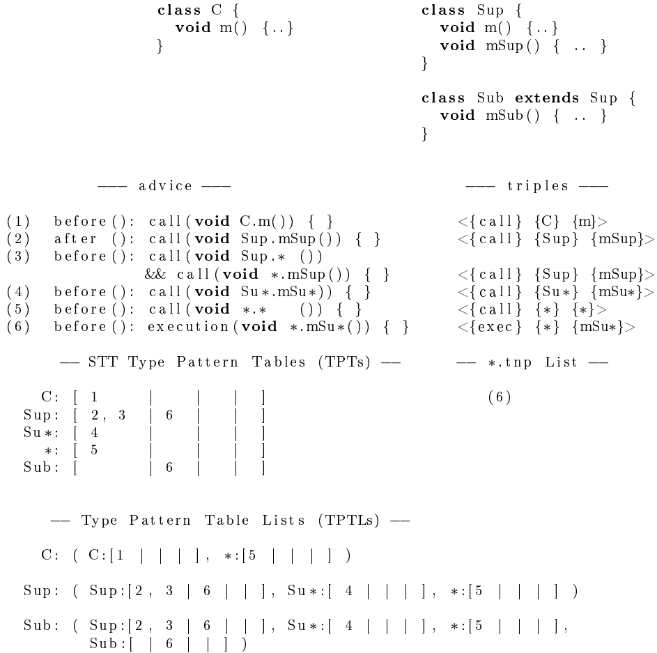
Figure 3.1: A simple example and the corresponding lookup table structures. The vertical bars divide the TPTs into four parts used to group advice by the kinds of DJPs they can match. Also note that advice 6 is added to the Sup and Sub TPTs during TPTL construction. The Sub TPT is created when the Sub TPTL is built.
