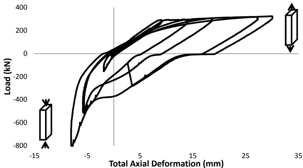
Figure 4-25 Axial load versus axial deformation for specimen C3
