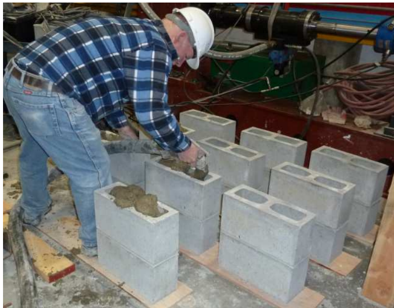
Figure 3-12 Construction of masonry prisms
