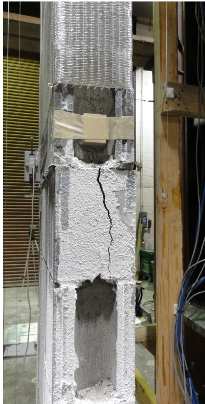
Figure 4-45 Large horizontal and vertical crack developed at the masonry course below the stiffened portion (above the 8th masonry course from base of the wall) of specimen C5 during load cycle #6 ( \Delta = 4.3\Delta_y )
