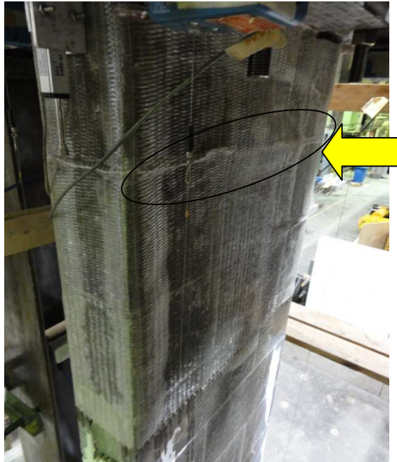
Figure 4-20 Open cracks underneath the GFRP overlay led to crushing of the overlay under compression loads (specimen C3)
