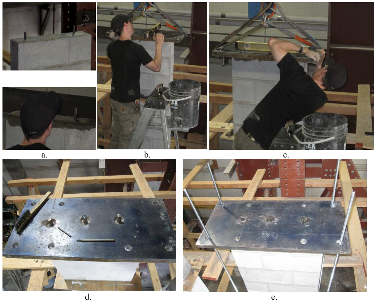
Figure 3-7 Welding of reinforcing bars to the top specimen plate
