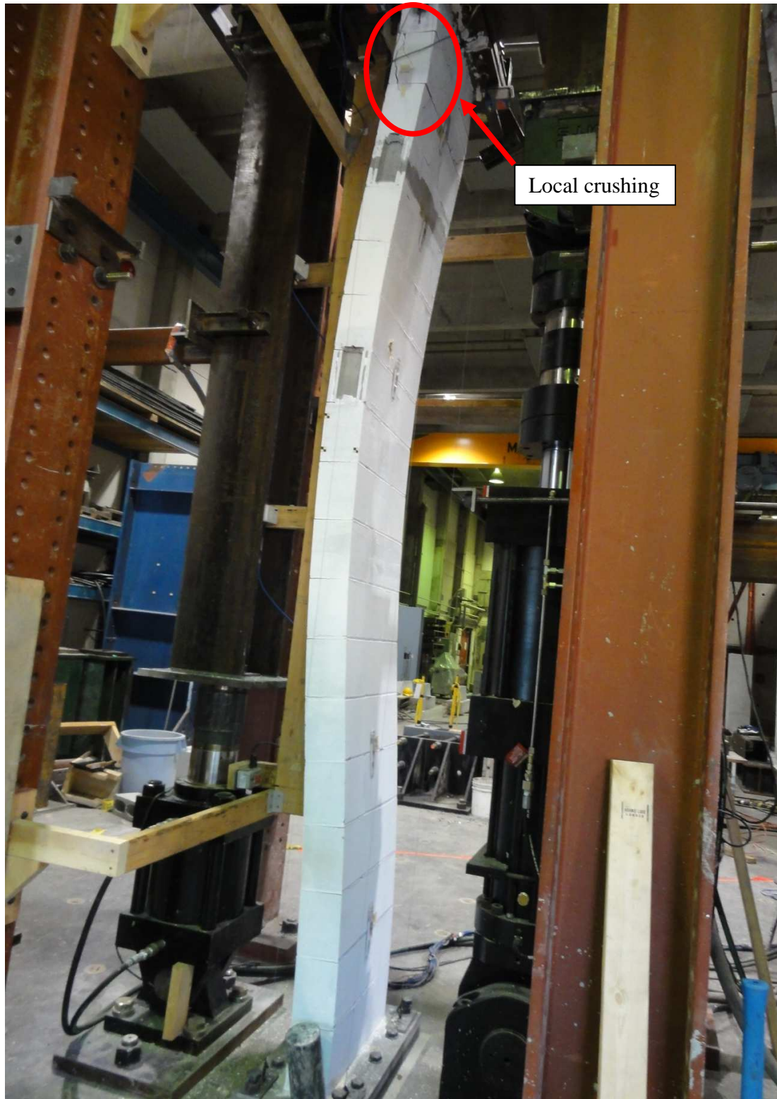
Figure 4-11 Specimen C2 at the end of the test, after experiencing out-of-plane instability
