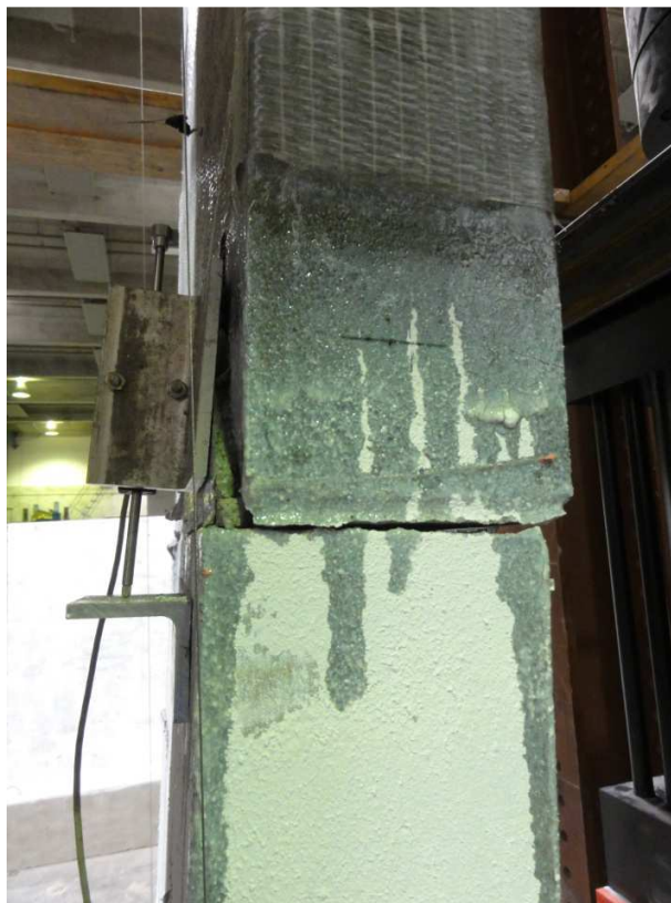
Figure 4-37 Sliding at the bed joint on the north face of specimen C4 at the ultimate stage
