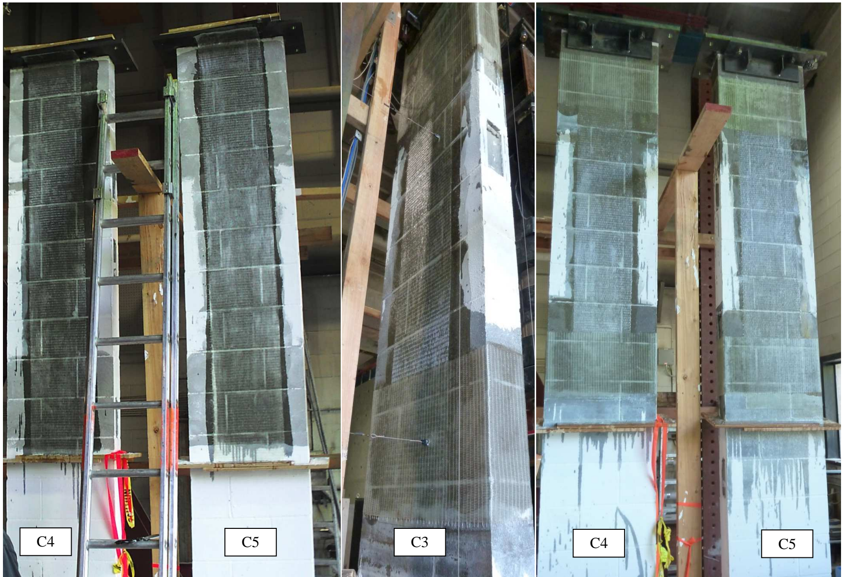
Figure 3-8 Application of GFRP over the top half of specimens C3 through C5
