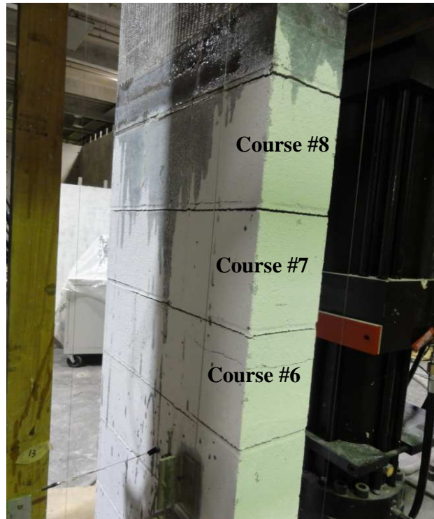
Figure 4-19 Horizontal cracks developed along all bed joints in the last tension cycle in specimen C3
