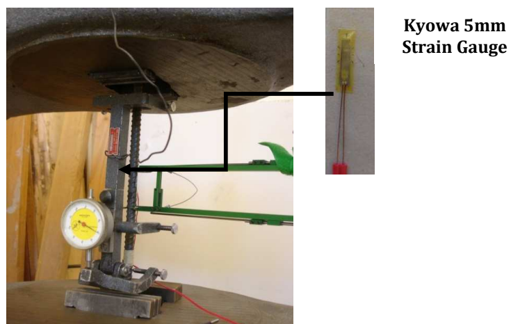
Figure 3-13 Testing reinforcement bars in the Baldwin universal testing machine
