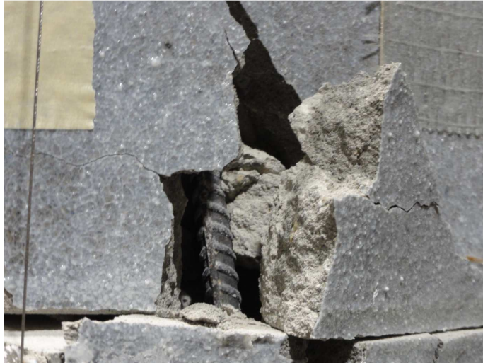
Figure 4-46 Reinforcing bar protruding through the block face shell during the compression half-cycle after the tensile axial displacement of 5.9\Delta y
