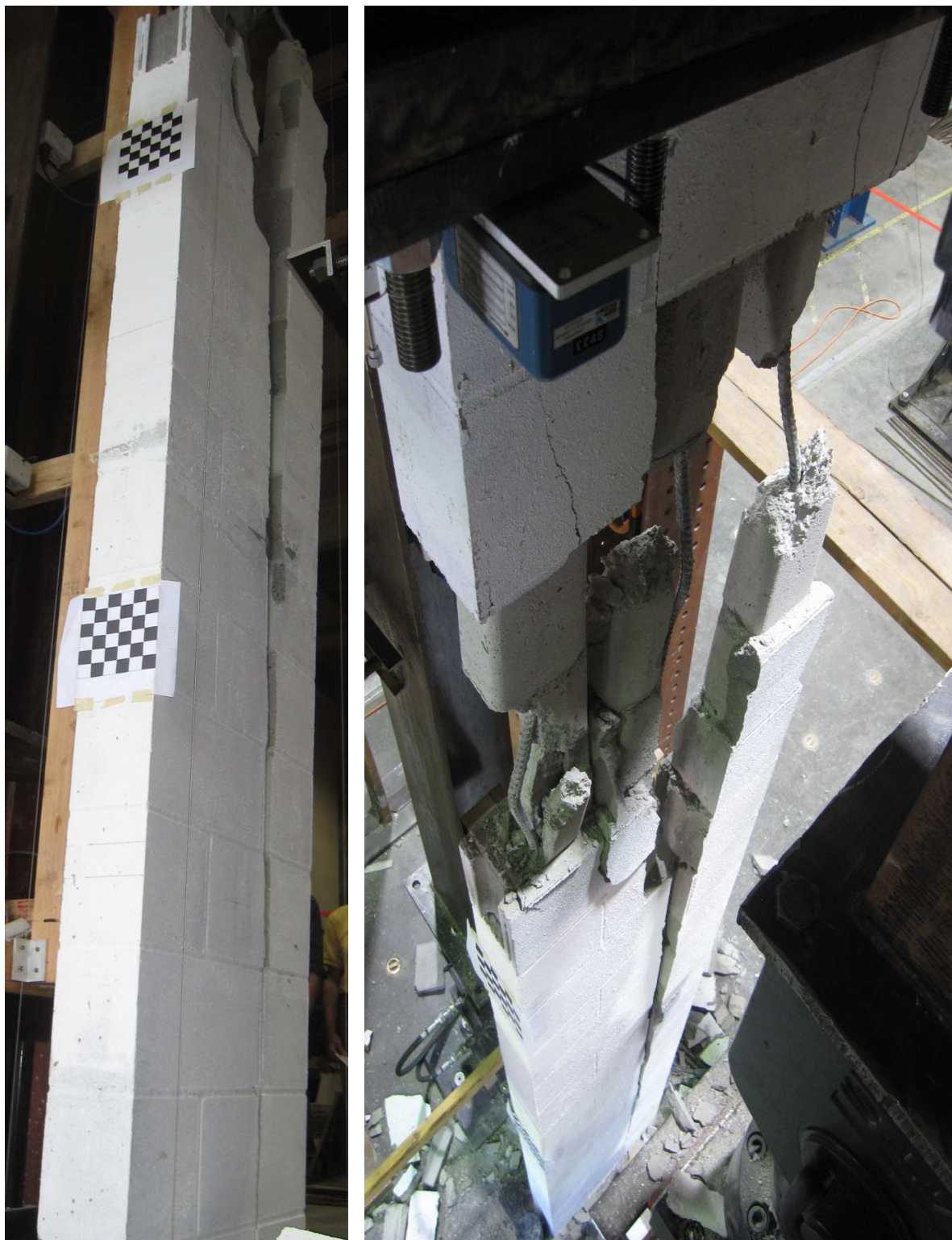
Figure 4-5 Specimen C1 at failure: note a continuous vertical splitting crack along the end block core (left) and disintegration of masonry in the crushed portion of the specimen (right)
