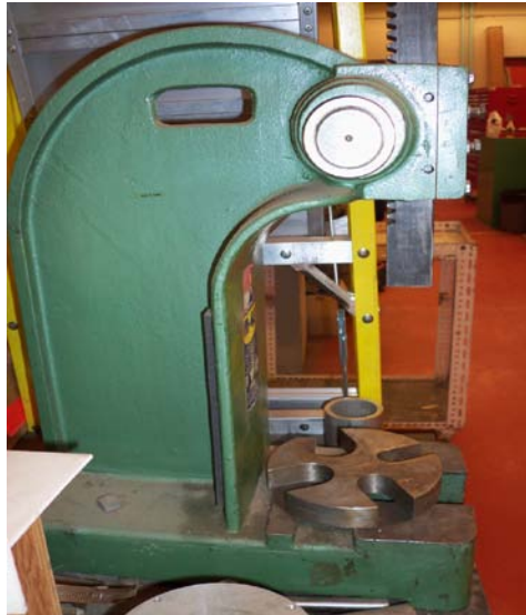
Figure B.1 Compression unit for soil static compaction.
