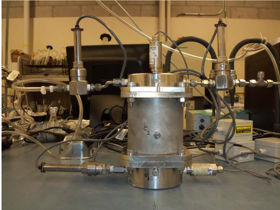
Figure 3.2 Effective diffusivity test apparatus (soil column).
