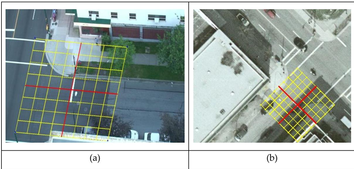
Figure 2.3 (a) Sample Grid on Image Space; and (b) Projected Sample Grid on World Space
