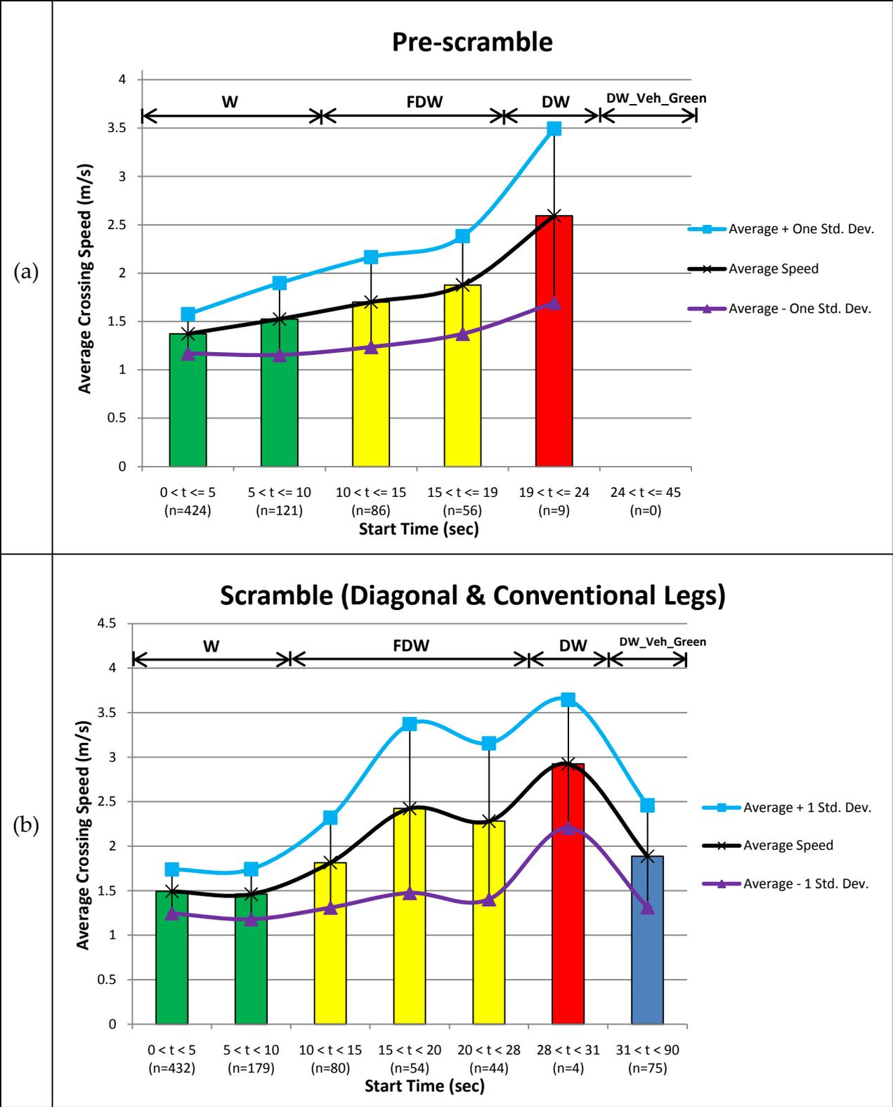
Figure 3.7 Pedestrian Walking Speed Behavior as a Response to Pedestrian Signal Indications
