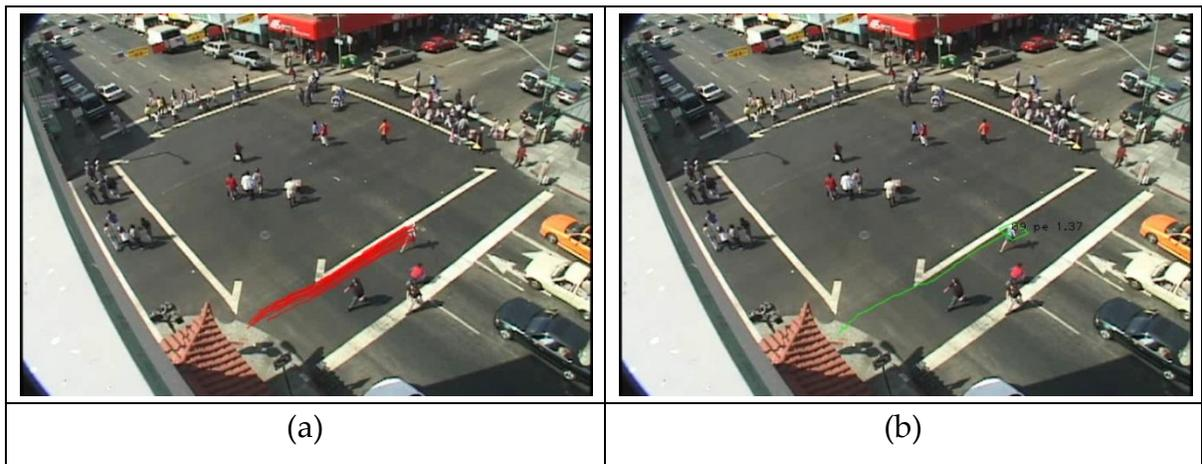
**Figure 2.1 Sample Pedestrian Tracking using Feature-based Tracking. (a) represents the detection of moving features and (b) represents a pedestrian object after grouping the features**
