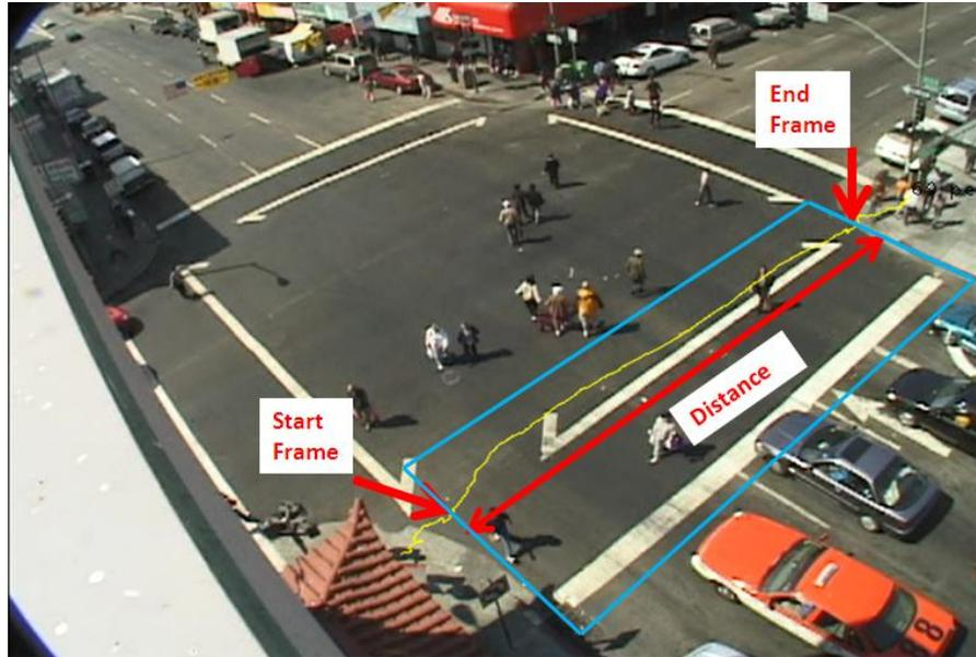
**Figure 3.3 Walking Speed Measurement Method**
