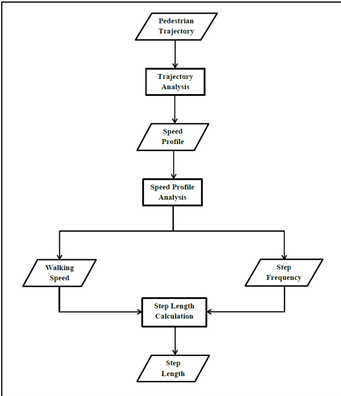
Figure 4.1 Pedestrian Gait Parameters Measurement Process
