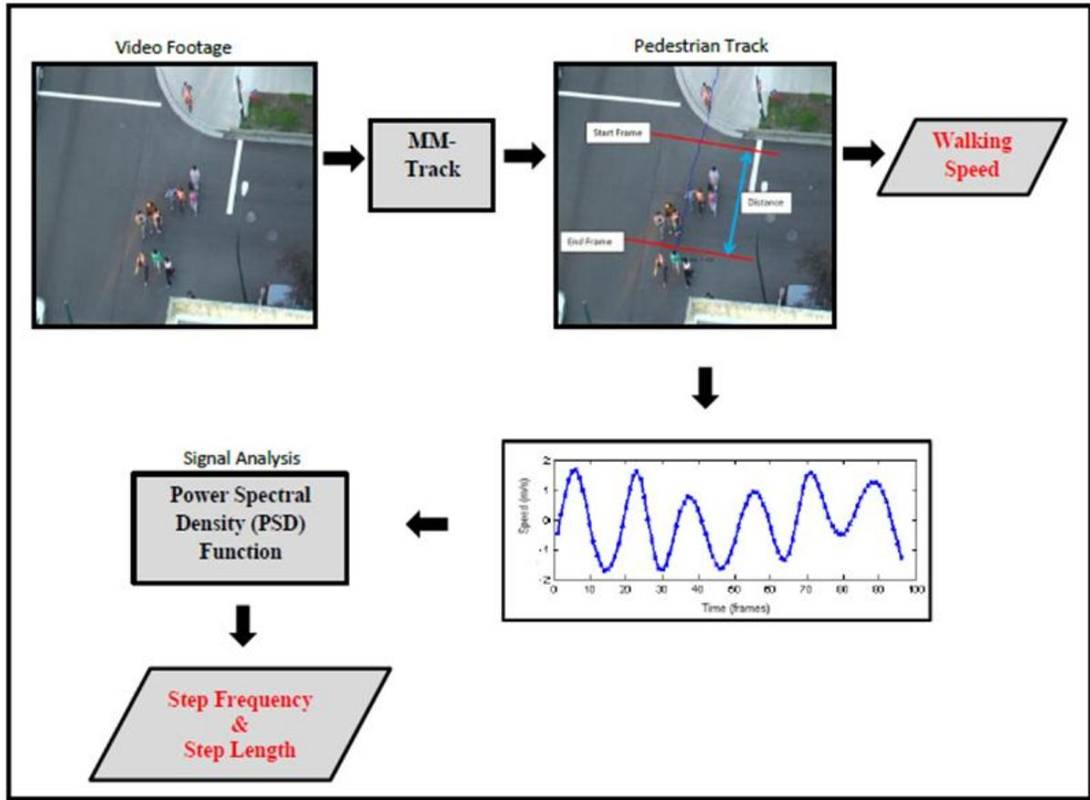
**Figure 4.2 Pedestrian Gait Parameters Measurement Method**
