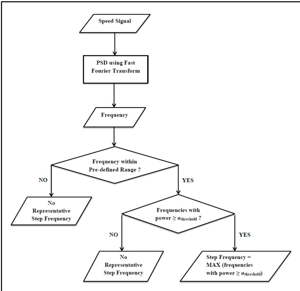
Figure 4.4 Walking Step Frequency Estimation Process
