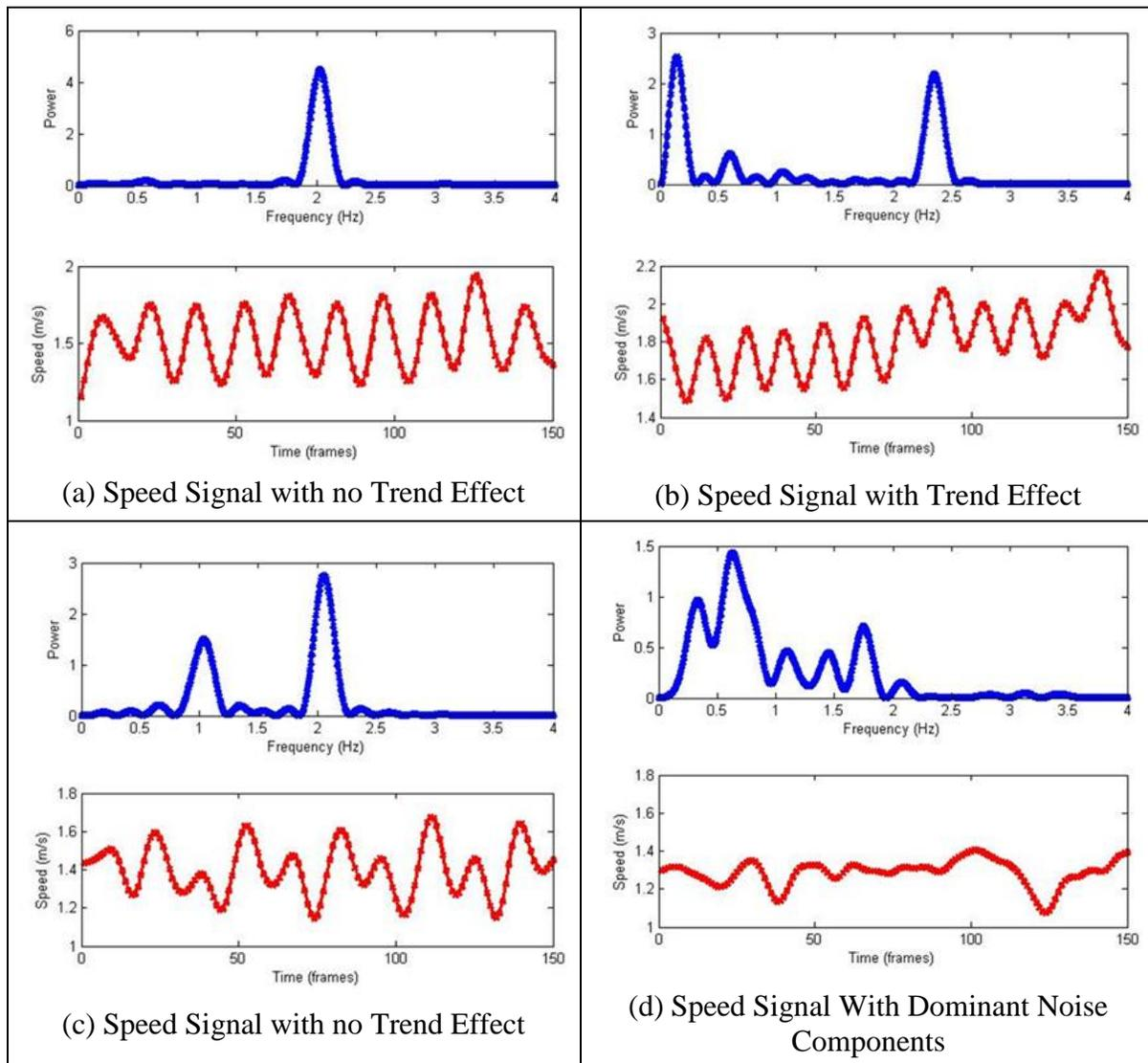
**Figure 4.13 Smoothed Pedestrian Walking Speed Signal (Bottom); Power Spectrum (Top)**
