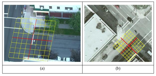
Figure 2.3 (a) Sample Grid on Image Space; and (b) Projected Sample Grid on World Space
