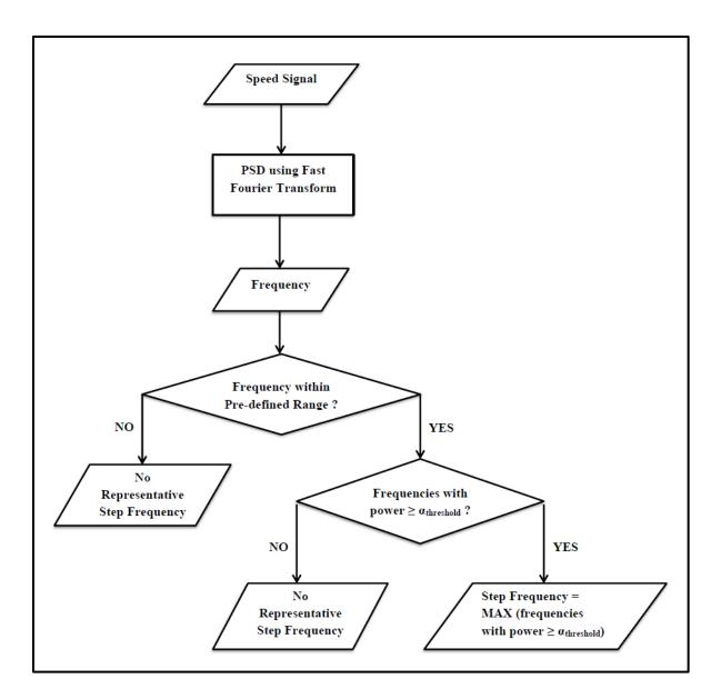
**Figure 4.4 Walking Step Frequency Estimation Process**
