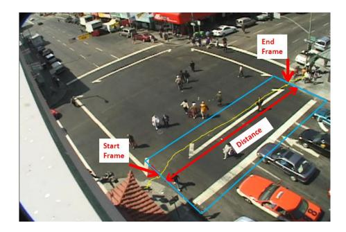
Figure 3.3 Walking Speed Measurement Method
