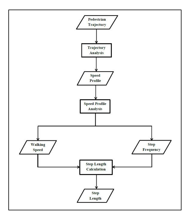
**Figure 4.1 Pedestrian Gait Parameters Measurement Process**
