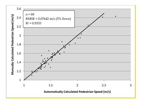
Figure 3.4 Comparison between Automatically and Manually Measured Walking Speeds in Scramble Phase
