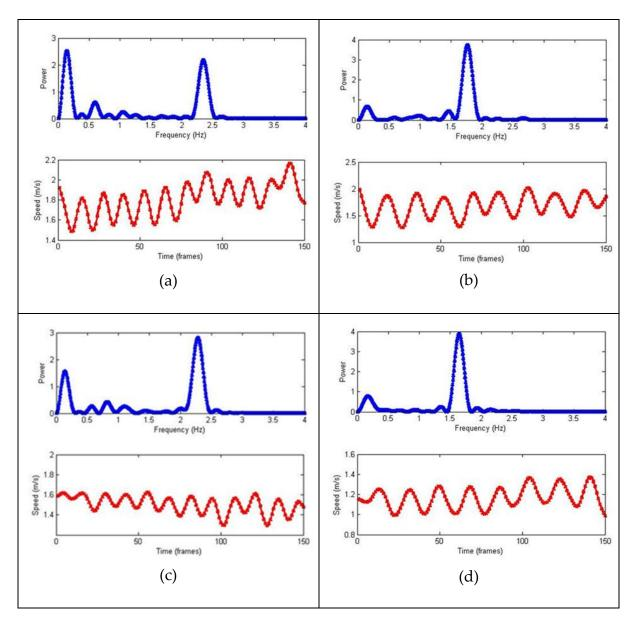
Figure 5.3 Pedestrian Step Frequency Estimation using Walking Speed Profile. (a) represents a Female subject aged between 36 and 55 with step frequency of 2.35 Hz; (b) represents a Male subject aged between 36 and 55 with step frequency of 1.76 Hz; (c) represents a Female subject aged between 17 and 35 with step frequency of 2.28 Hz; (d) represents a Female subject aged over 55 with step frequency of 1.65 Hz
