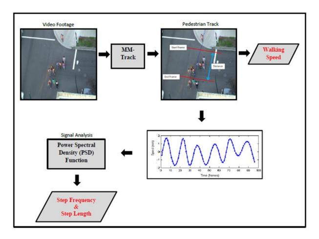
Figure 4.2 Pedestrian Gait Parameters Measurement Method
