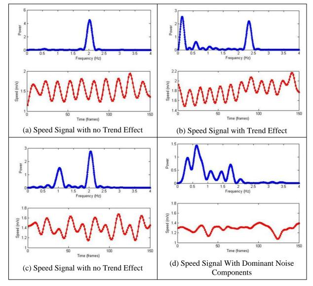
Figure 4.13 Smoothened Pedestrian Walking Speed Signal (Bottom); Power Spectrum (Top)
