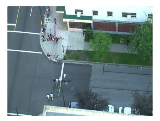
Figure 4.7 Vancouver Case Study Intersection Layout and Sample Pedestrian Tracks
