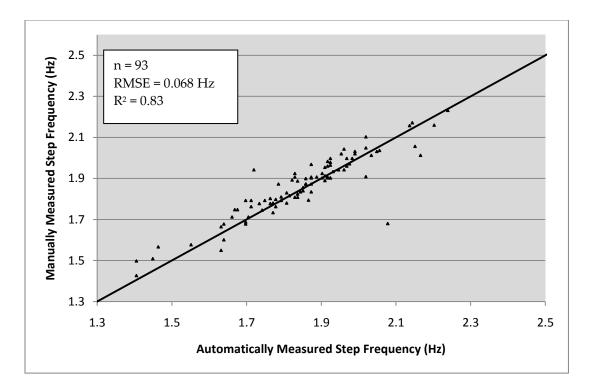
Figure 4.5. Comparison between Automatically and Manually Measured Pedestrian Step Frequencies
