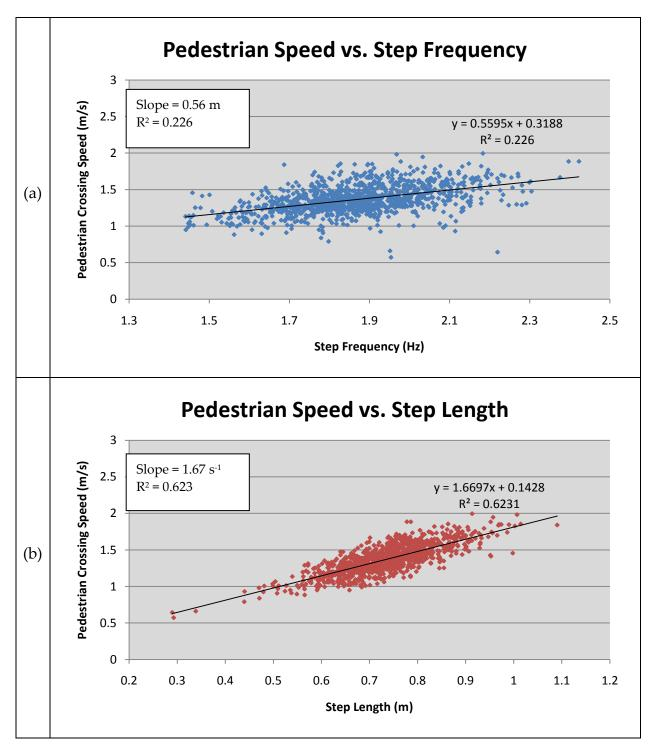
Figure 4.8 Effect of Pedestrian Step Frequency and Step Length on Walking Speed
