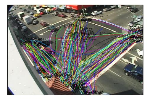
Figure 3.2 Sample Object Tracks in Scramble Phase with 8 Seconds or Longer Duration of Detection
