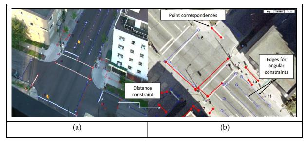
Figure 2.2 Calibration Data. (a) Image Space; (b) World Space. Source: (Ismail, et al., 2010)
