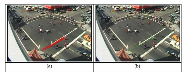
Figure 2.1 Sample Pedestrian Tracking using Feature-based Tracking. (a) represents the detection of moving features and (b) represents a pedestrian object after grouping the features
