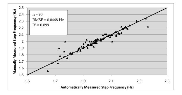
Figure 4.14 Comparison between Automatically and Manually Measured Pedestrian Step Frequencies
