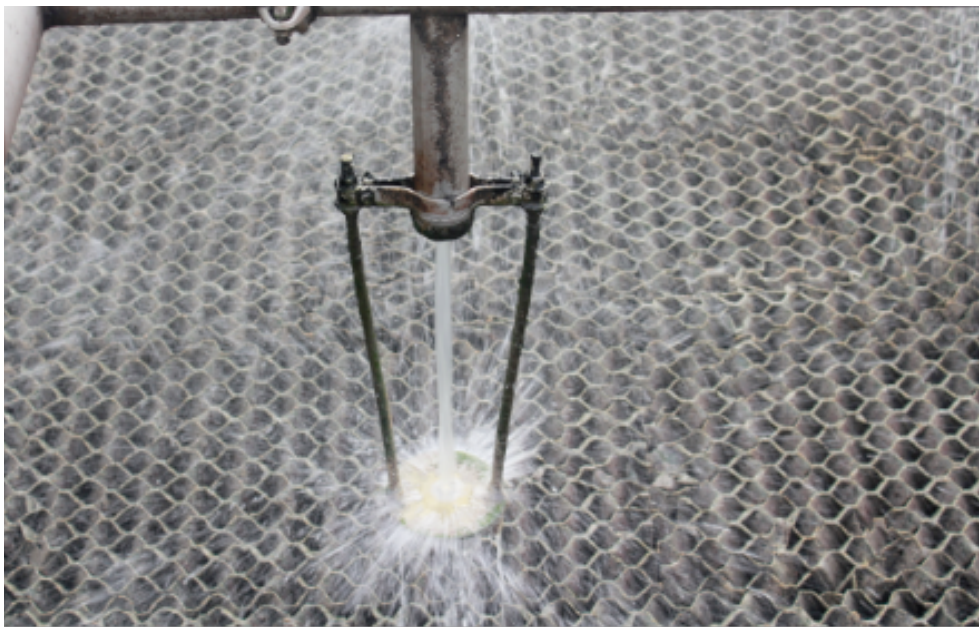
Figure 2.7 Close up of water distributor and trickling biofilter media
