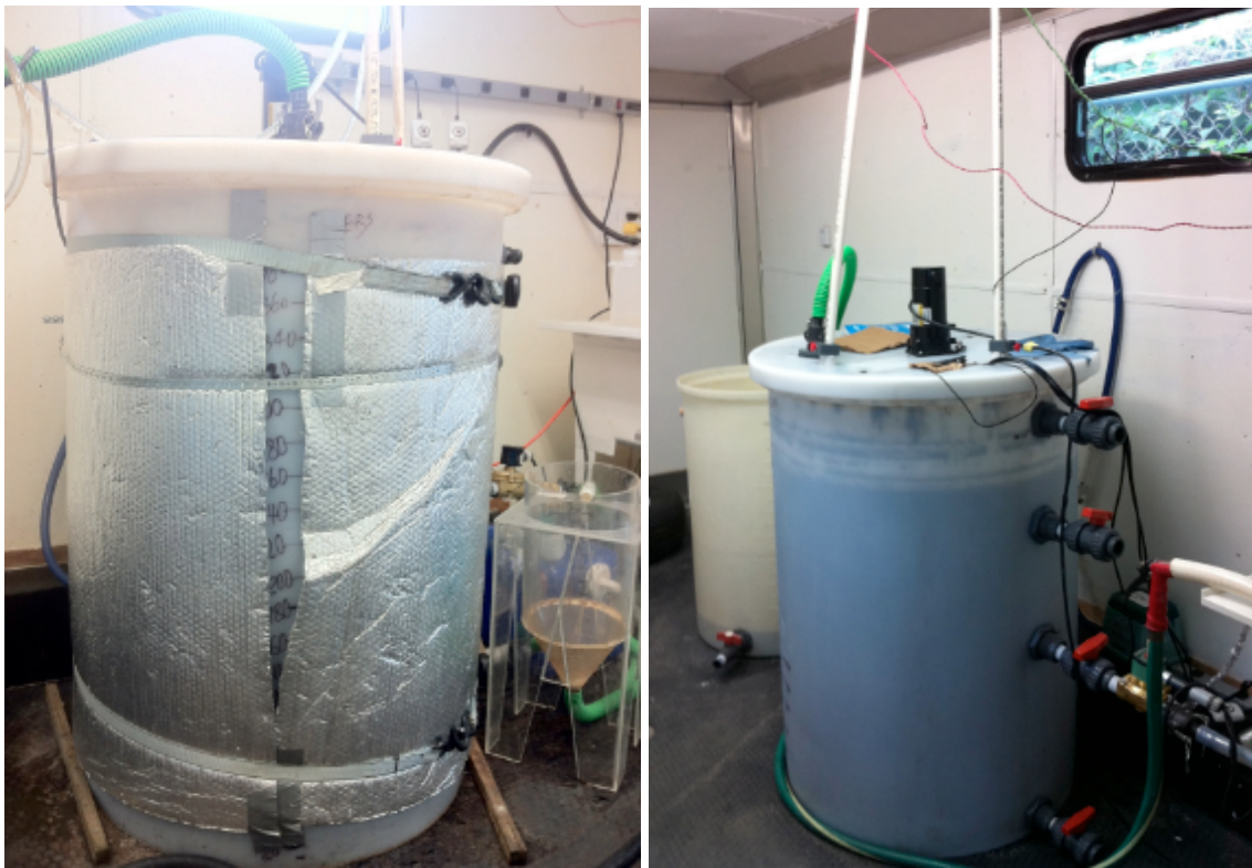
Figure 2.15 Sequencing batch reactor (SBR) for the CANON process
