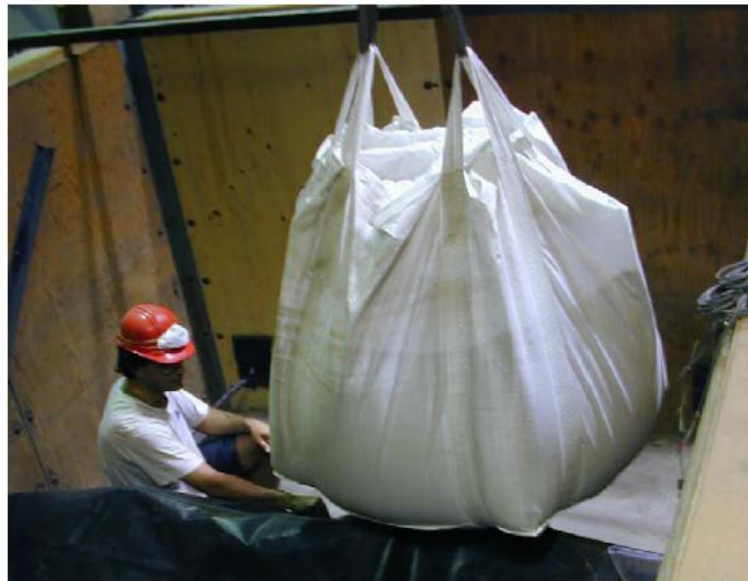
Figure 3-20: Loading preparation phase, bulk bag suspended by overhead crane.
