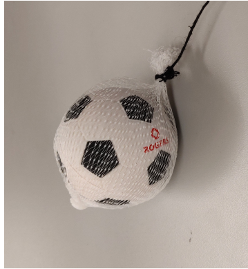
(a) Photo of 18g Mock Bird Used for Validation Tests
