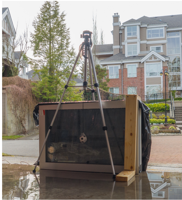
Figure E3: Full Rain Test Setup
