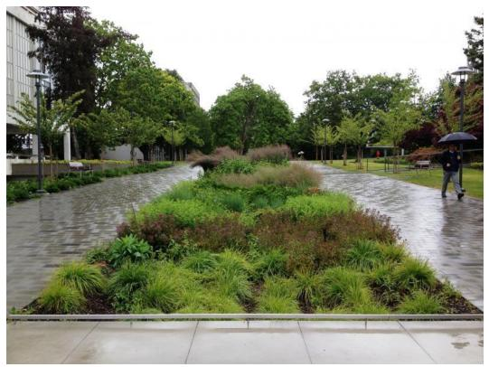
*Figure 9 Example of a rain garden showcased at UBC* Source: planning.ubc.ca, Turning Rainfall into a Resource
