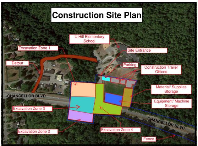
Figure F - 1 - Construction Site Plan
