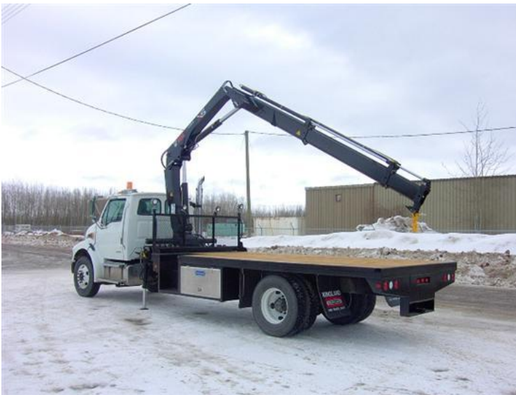
Figure 4 – Transportation Vehicle with Mounted Crane
