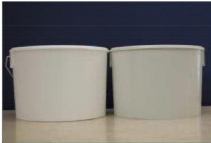
Figure 1 – Color comparison of recycled polypropylene and virgin polypropylene
