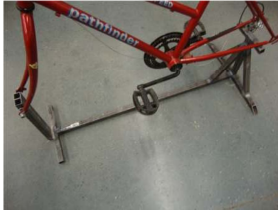
Figure 4: New Bike Support Structure
