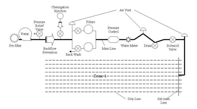
Figure 1. A comprehensive drip irrigation system
