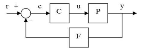
Figure 6. Closed-loop Feedback System Source: Wikipedia – control theory
