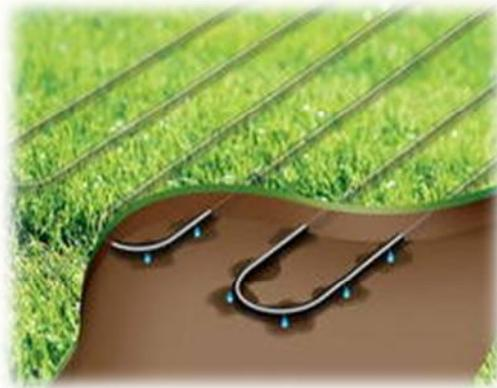
**Figure 6 :** Cut away diagram of sub irrigation drip tape
