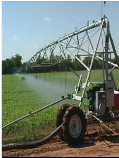
**Figure 12:** Lateral Move Irrigation
