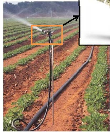
**Figure 13:** Impact Sprinkler Irrigation
