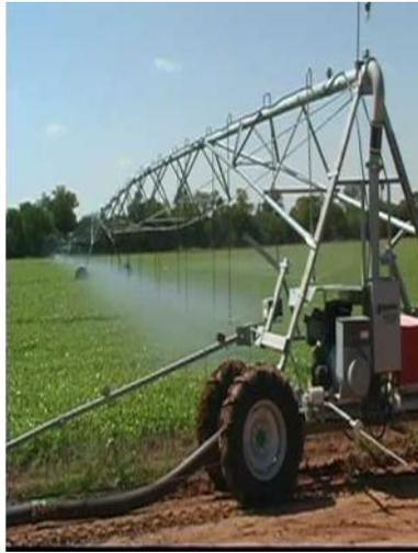
**Figure 12:** Lateral Move Irrigation
