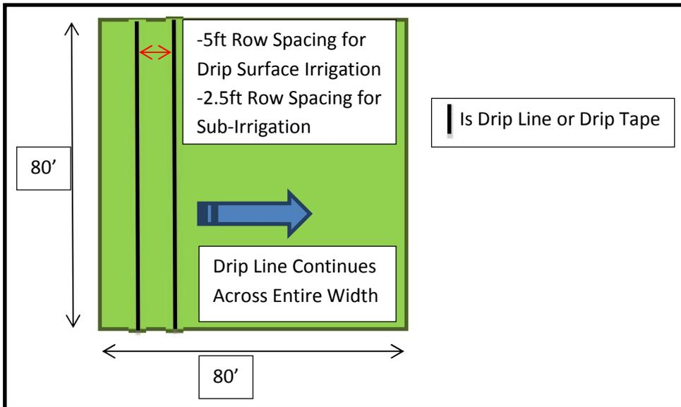
**Figure C2 - Set Up for Drip Line Surface Irrigation and Sub-Irrigation**
