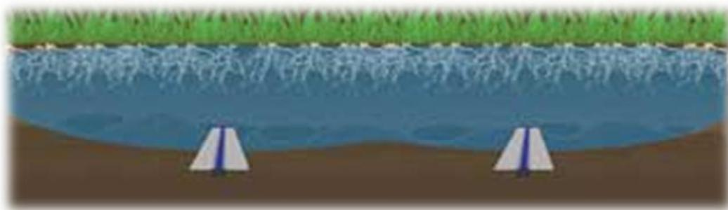
**Figure 7 :** Wetting pattern of soil above sub irrigation drip tape
