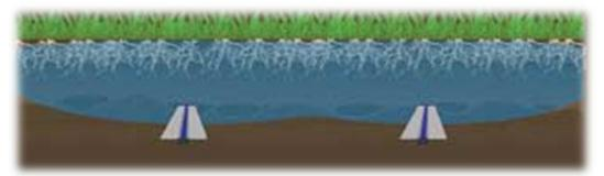
Figure 7 : Wetting pattern of soil above sub irrigation drip tape Source: http://www.fao.org
