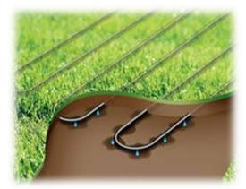
Figure 6 : Cut away diagram of sub irrigation drip tape Source: http://www.dwc-water.com
