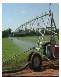
Figure 12: Lateral Move Irrigation Source: <u>www.centerirrigation.com</u>
