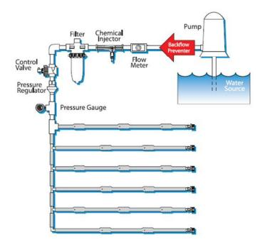
**Figure 4** : Typical layout of a drip irrigation system Source: <u>http://www.dripirrigation.org/images/ALT142\_What%20Is%20Drip%20article\_WEB.pdf</u>
