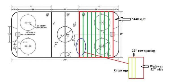
Figure X: Possible setup of the drip irrigation system. Source: http://cdn.nhl.com/images/upload/2008/06/rink\_diagram.gif
