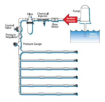
Figure 4 : Typical layout of a drip irrigation system
