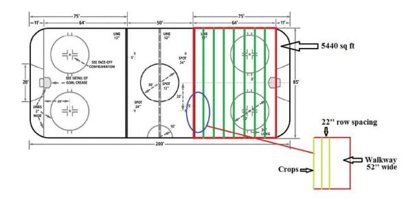
Figure X: Possible setup of the drip irrigation system.
