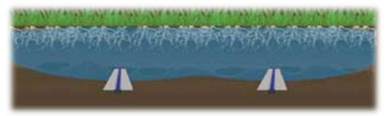
**Figure 7 :** Wetting pattern of soil above sub irrigation drip tape Source: http://www.fao.org
