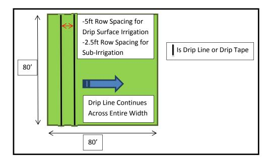
Figure C2 - Set Up for Drip Line Surface Irrigation and Sub-Irrigation
