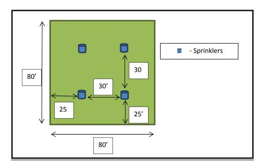
Figure C1 - Sprinkler Irrigation Set-Up for Calculations
