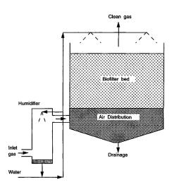
Figure 1: An open Biofilter
