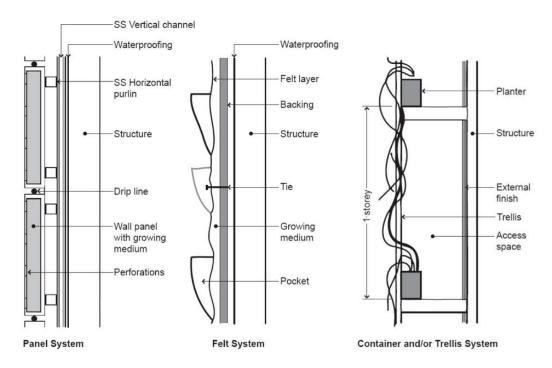
Figure 3: Three Biowall Structure Examples
