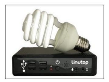
FIGURE 2: LINUTOP NETTOP AND A CFL BULB FOR COMPARISON OF SIZE AND POWER USAGE (8w)
