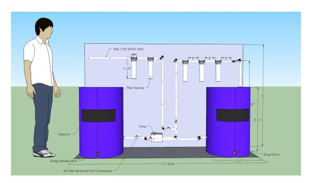
Figure 2: Front View with Dimensions
