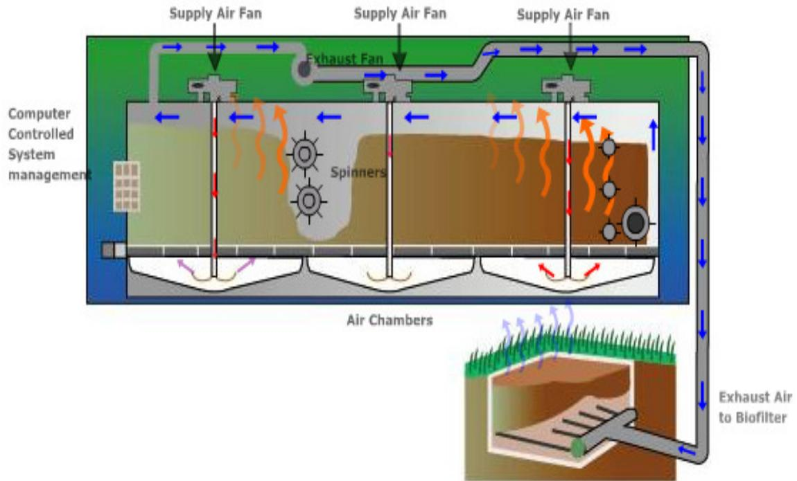
**Figure 7: In-vessel Compost Diagram**
