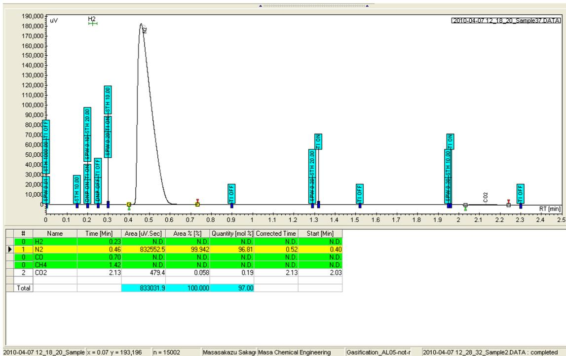
Figure 6: Gas Chromatography Analysis in Bio-Filter Sample 2
