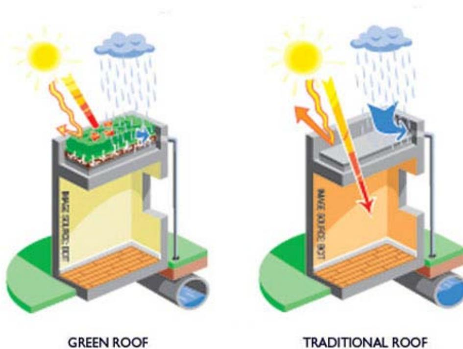
Figure 1: Rooftop Gardens can reduce the energy needed for cooling or heating the building.
