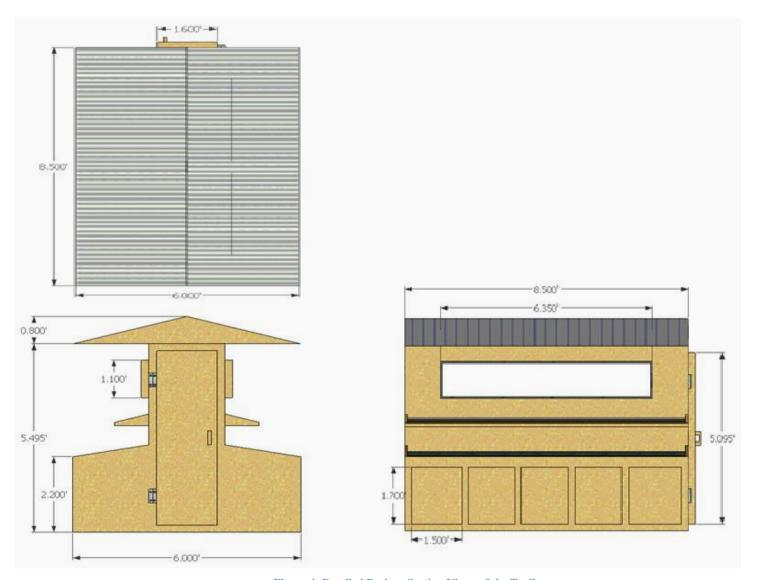
Figure 4: Detailed Design: Section Views of the Trailer
