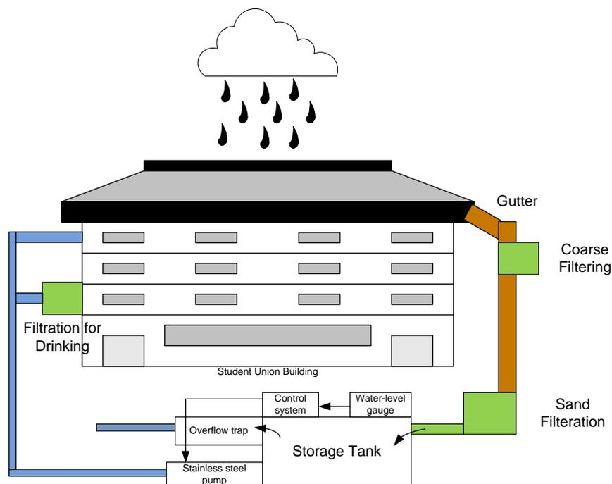
*Figure 4: Rainwater harvesting system block diagram*
