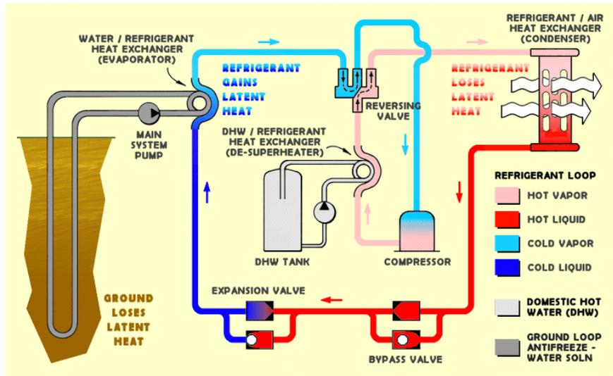
Figure 1: Geothermal Heating Schematic<sup>3</sup>
