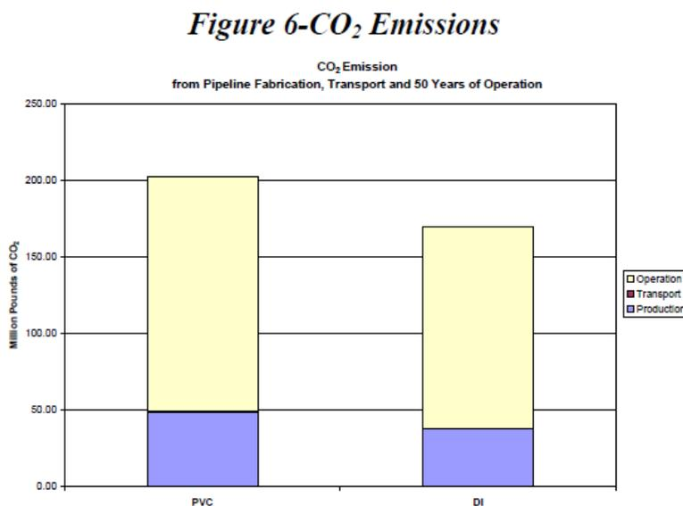
Figure 4 Ecological Footprint of PVC vs. DI
