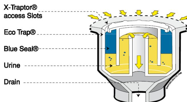
**Figure 3: non-flush Eco-Trap system**
