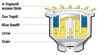
Figure 3: non-flush Eco-Trap system
