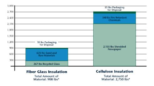
Figure 1 - Waste content of packaging cellulose fibres vs. fibreglass insulation, Source: NAIMA (2009)
