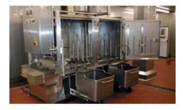
Figure 2 – Bin Washer System from Industrial Washing Machines
